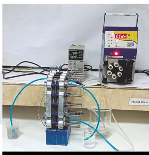
Hydrogen is produced at a rate of one litre per hour when a large electrolyser is used
